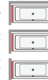
**FILLER PANELS:** the peninsula, corner and niche types require the use of the EPS panel provided (P3) to be installed on the smaller side against the wall.
